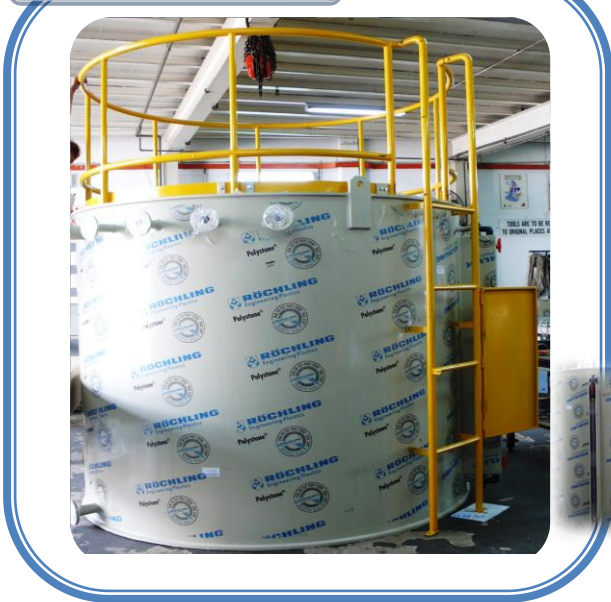
PP VESSEL TANK
